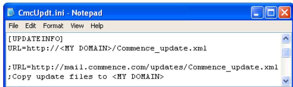
Figure 2-5: Sample changes to configuration file
